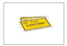
CL... caution labels are vinyl-based peel and stick, with black letters on a yellow background, and are intended for direct exposure to industrial environments. Local codes and standards require electrically heated pipelines and vessels to be clearly identified "at frequent intervals along the pipeline or vessel." Caution labels should be placed at 3-6 m intervals or as required by code or specification.
