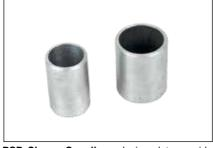
**PSP Sleeve Coupling...**designed to provide the correct size coupling to connect the boxes to the heat tube and each heat tube together. Each coupling is 50 mm long and has been deburred and chamfered at the factory.
