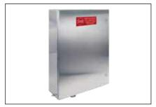
**PSP Field Junction Box...** is a stainless junction box designed to be placed between the control panel and the on-the-pipe power box. This allows connection of power to the circuit of the pipe outside of the high temperature environment, and easy access for disconnecting the circuit during maintenance. Rated for ATEX/ IECEx, Ex eb, Ex tb, IP66, up to 5000V. 914 x 610 x 203 mm.
