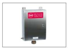
**PSP External Splice Box...** a stainless junction box designed to make splice connections outside of the insulation for high temperature applications. Rated for ATEX/IECEx, Ex eb, Ex tb, IP66, up to 5000V. 406 x 305 x 152 mm.
