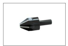
Countersink 6 Flute... designed to deburr and chamfer the ends of all heat tubes. Features six flutes to reduce chattering. Shank diameter is 12.7 mm.
