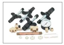
Heat Tube Air Test Kit... designed to ensure that all heat tube field weld joints are structurally and electrically sound. Kit includes pressure gauge and fits both ¾" and 1" heat tube.
