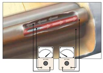
AC voltage will generate a current in the conductor which returns through the inside surface of the heat tube. There is virtually no measurable voltage on the outer surface of the heat tube, allowing the piping system to be grounded.
